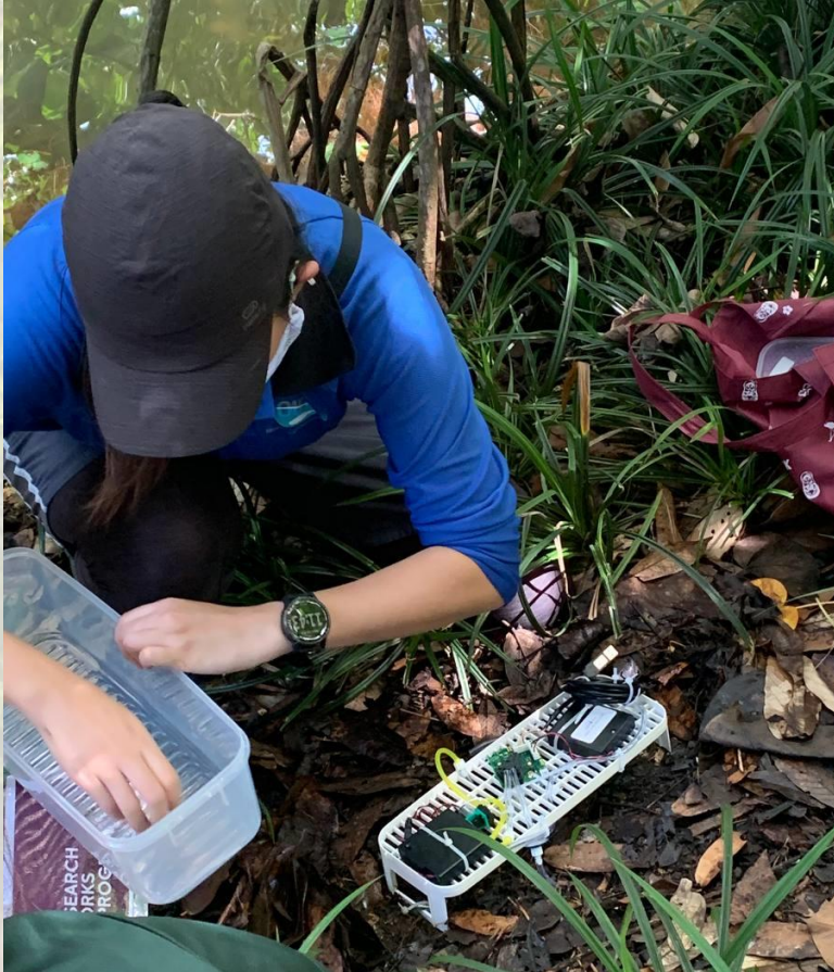
Soil gas flux: to measure \text{CO}_2 due to autotrophic and heterotrophic activity in the sediment
