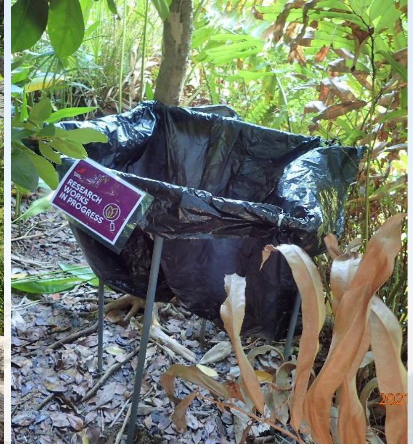
Leaf litter trap: Measurements of organic carbon content (autochthonous carbon) in leaf litter
